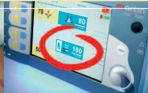
Fig. 3: A typical setting selected on the maxium® HF generator for the sealing procedure illustrated on the left (Fig. 1).
